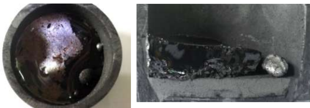
Fig 4 : Top and section view of graphite crucible with glassy slag and pig iron produced from red mud reductive smelting
