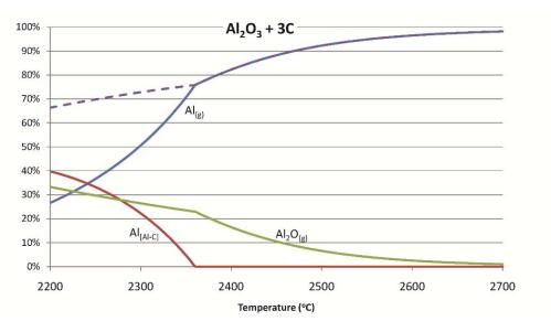
**Figure 2:** Factsage calculated distribution of aluminum species at thermodynamic equilibrium for various temperatures at atmospheric pressure in a system with initial molar composition of  $1 \text{ Al}_2\text{O}_3 + 3 \text{ C}$ . The dashed line signifies the total alumina to metallic aluminum reduction yield (AI-C alloy and  $\text{Al}_{(g)}$ ). The [AI-C] subscript denotes the liquid aluminum alloy metal phase.
