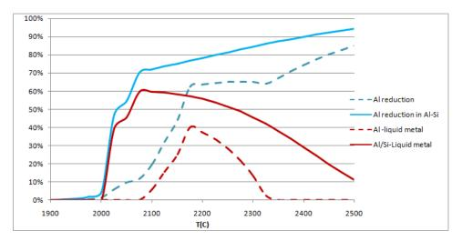
**Figure 5**: Prediction of aluminium overall reduction rate and aluminium liquid metal recovery rates for the system  $2 \text{ Al}_2\text{O}_3 + 1 \text{ SiO}_2 + 8 \text{ C}$  (solid lines) and the system  $\text{Al}_2\text{O}_3 + 3 \text{ C}$  (dashed lines).
