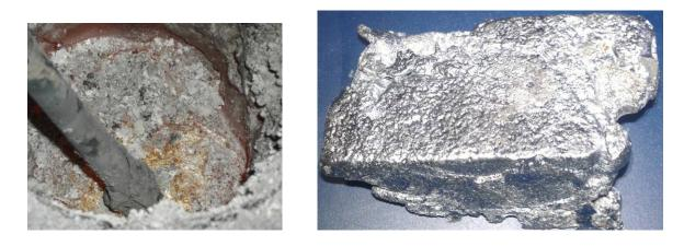
**Figure 6** - **Left:** Visible aluminium melting "skin" during solidification process of the melt, **Right:** Picture of the casted carbothermically produced AI-Si alloy.
