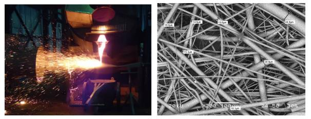
**Figure 1:** Photos of air/water jet slag fiberization test (left) SEM photograph of inorganic fibers produced (right).
