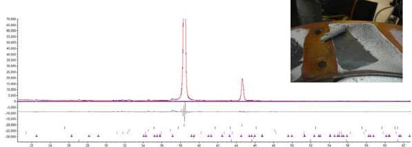
**Figure 4:** XRD analysis of the dust collected from the condenser. Both major picks correspond to metallic aluminium (2theta 38,10 and 44.37). Rietveld-method analysis shows at least 76.91% metallic AI, followed by cubic Alumina 9.37%, 4% or less in  $Al_2OC$ ,  $Al_4C_3$  and  $Al_4O_4C$ . Cubic alumina is the result of metallic aluminum re-oxidation after the end of the experiment. **Inlet Picture:** Dust collected from copper condenser surface.
