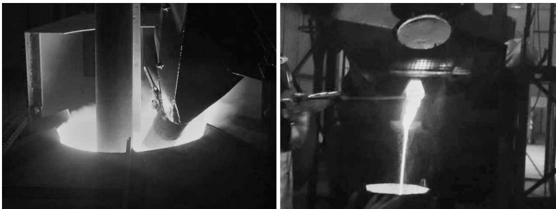
Figure 4: Photos of the EAF during batch feeding (left) and during pouring (right)
