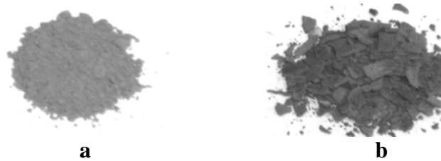
Fig.7 Powders from place 3a with 59% of pure aluminum (a) and from place 7 with 98% of pure zinc (b)
