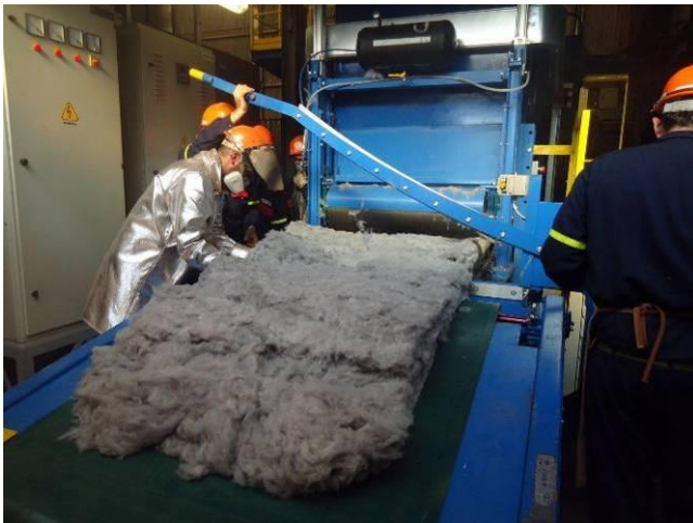
Figure 6. Production of mineral wool fibers from BR-slag in the AoG pilot plant
