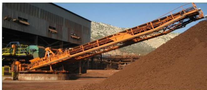
Figure 1. Dewatered BR exiting the filter presses in AoG
