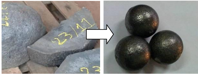
Figure 5. Produce Pig-iron ingots (left) and respective white iron grinding balls from Guca foundry in Serbia (right), produced with up to 21%wt steel scrap substitution from BR-pig iron (ball diameter: 70 mm, ball composition: Fe 92.7% wt, Cr 2.81%wt, Si 0.51% wt, S 0.05%/ wt, P 0.07%wt ).
