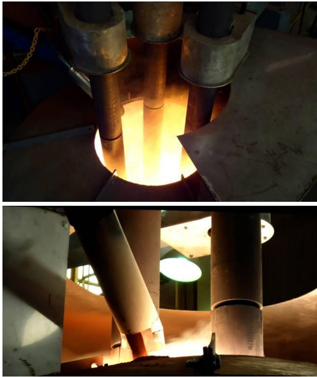
Figure 3. Photographs of the continuous feeding of the EAF with the dusty material mix, through a top lance feeder in the AoG pilot plant.
