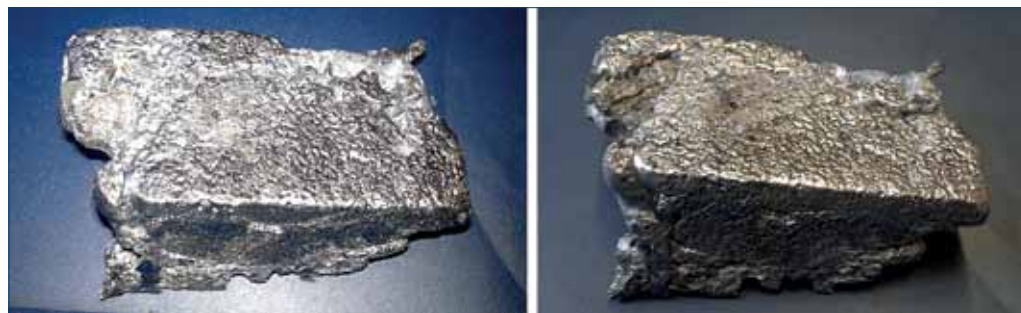
Fig. 13: Pictures of carbothermally produced Al-Si alloy in experiment 10
