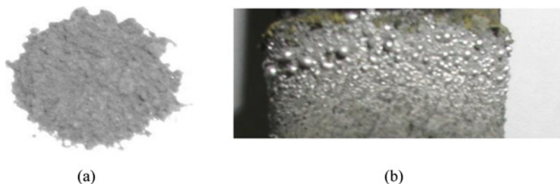
Figure 2. Example of deposits: (a) powder with 70% Al scraped from inner surface of zirconia tube and (b) aluminum drops condensed on molybdenum tube with OD = 20 mm (color figure available online).
