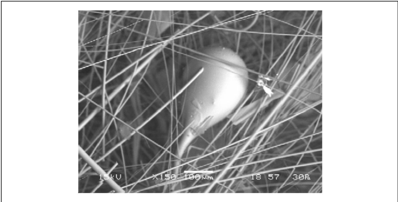
Figure 7: SEM photograph of inorganic fibres produced from the red mud treatment process slag, magnification 150×
