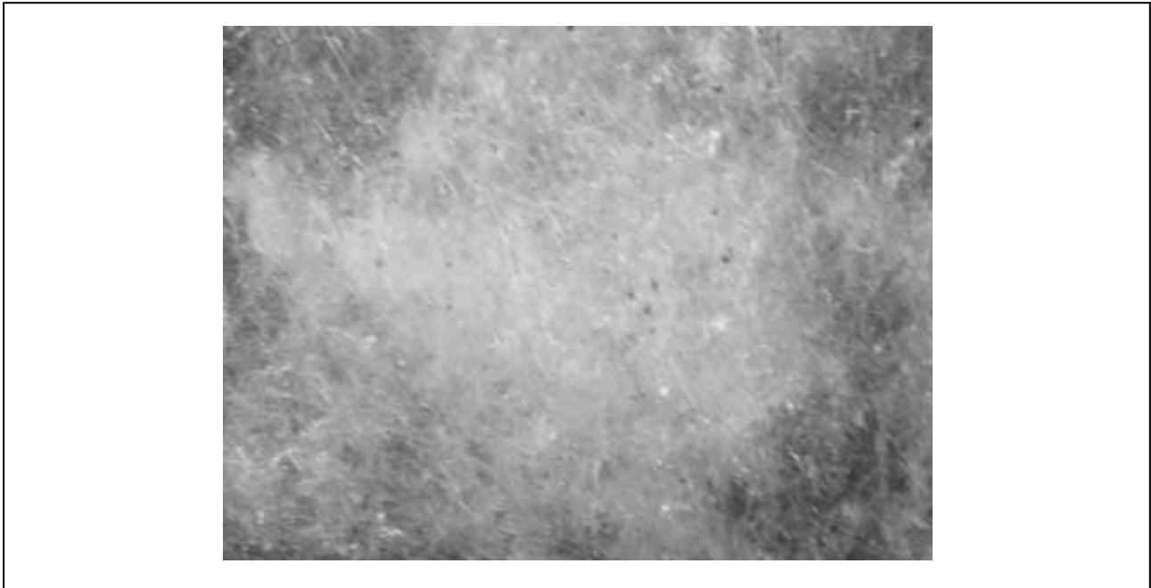
Figure 5: Photograph of inorganic fibres produced from the red mud treatment process slag
