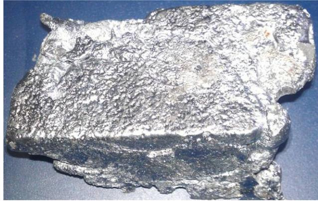
**Figure 6 - Left:** Visible aluminium melting “skin” during solidification process of the melt, **Right:** Picture of the casted carbothermally produced Al-Si alloy.
