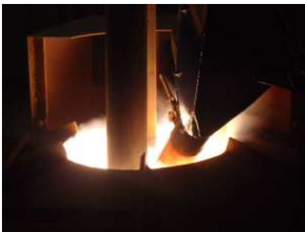
Figure 2: Photos of the EAF during batch feeding (left) and during pouring (right).
