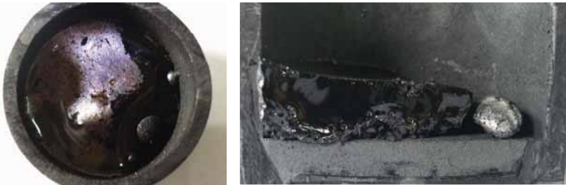
Figure 3: Top and section view of graphite crucible with glassy slag and pig iron produced from red mud reductive smelting (NTUA)
