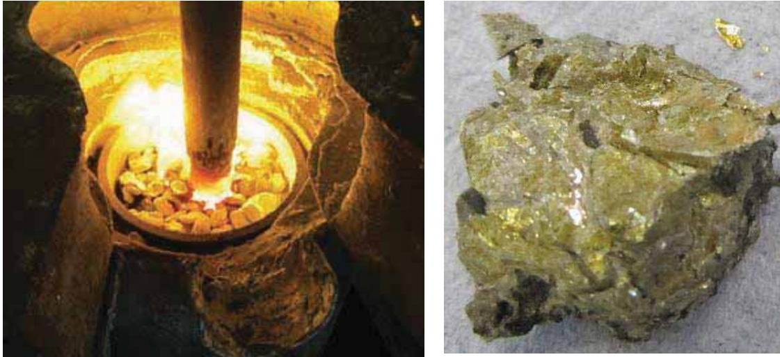
Figure 1: EAF experiments for the carbothermic reduction of alumina and produced aluminium-carbon alloy (RWTH-Aachen).
