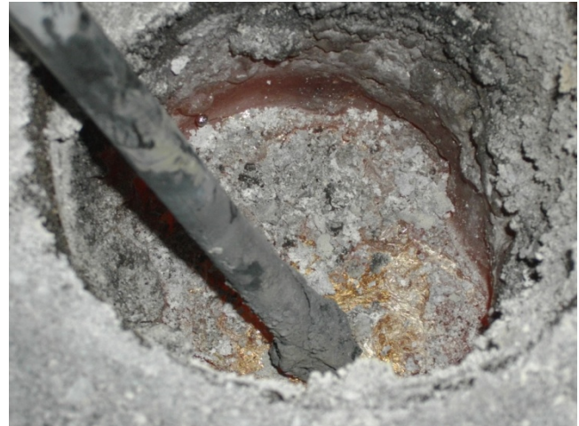
Figure 8: Photograph of produced Al-Si Melt and with characteristic “aluminum skin”
