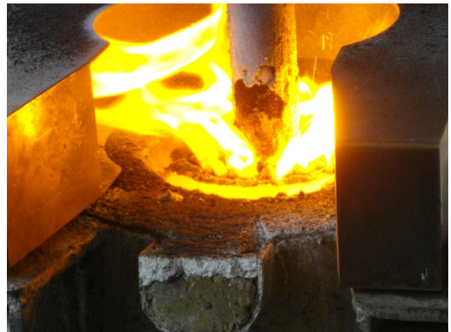
Figure 6: Furnace operation and Melt Sampling
