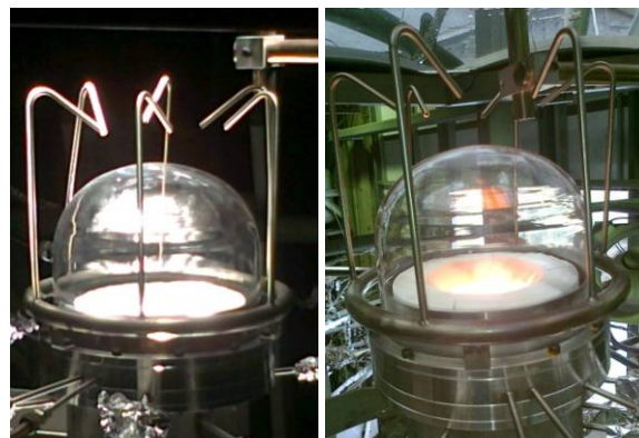
Figure 7. Solar reactor in operation (left) and cooling after operation (right)
