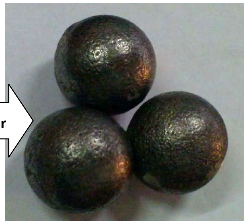
Figure 3 - Above: Red mud treatment process pilot plant in operation (ALSA); Below Right: produced pig-iron ingots; Below Left: End product, white cast iron balls 70mm, produced using pig-iron from the ALSA plant as scrap substitute.
