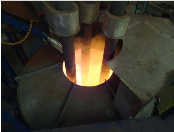
Figure 3 - Above: Red mud treatment process pilot plant in operation (ALSA); Below Right: produced pig-iron ingots; Below Left: End product, white cast iron balls 70mm, produced using pig-iron from the ALSA plant as scrap substitute.
