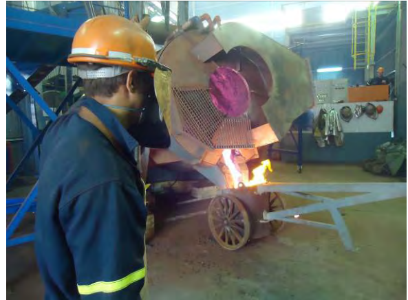
Figure 3 - Above: Red mud treatment process pilot plant in operation (ALSA); Below Right: produced pig-iron ingots; Below Left: End product, white cast iron balls 70mm, produced using pig-iron from the ALSA plant as scrap substitute.
